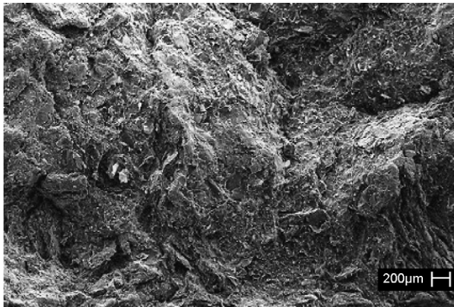
Fig. 16. SEM of the fractured surface of the composite plate without fiber content.
